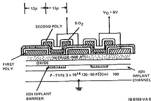
Figure 2. Cross Section of CCD-321 Structure
