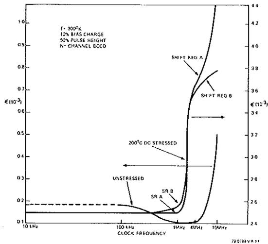
Figure 6. Transfer Efficiency versus Clock Frequency for BCCD's
