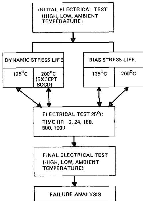
Figure 3. Life Test Plan for CCD Devices
