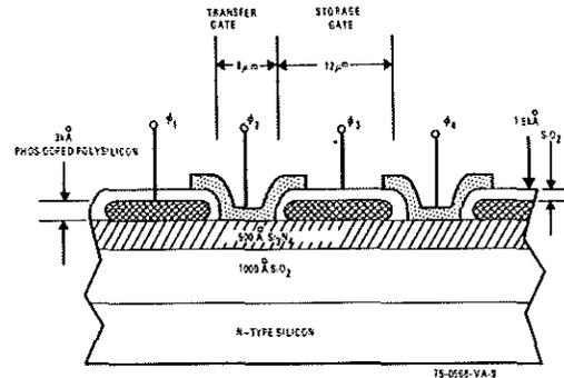
Figure 1. Cross Section of Aluminum/Poly Silicon Four Phase, Coplanar Electrode Configuration
