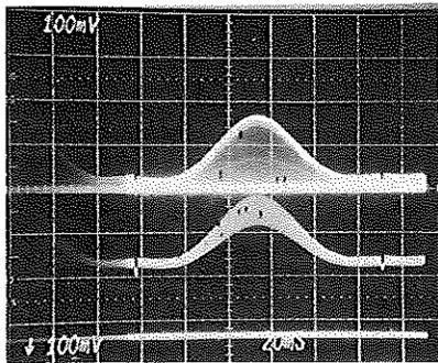
Fig. 4 Transversal Filter Impulse Response,  $f_c = 1.0 \text{ kHz}$
