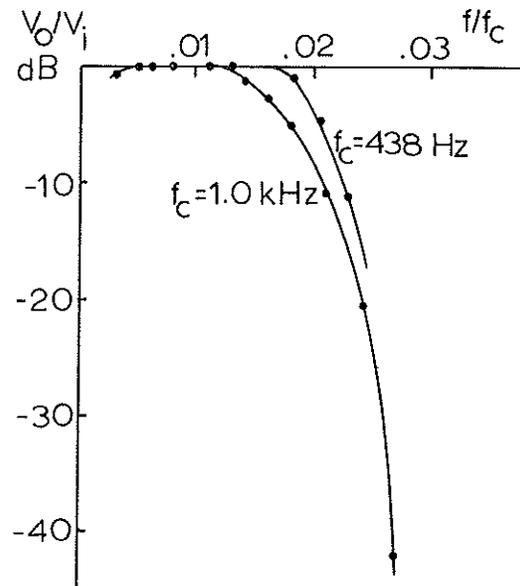
Fig. 5 Measured Frequency Response of the Transversal Filter
