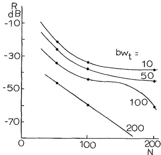
Fig. 2 Narrow Band Filter Design Curves
