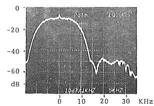
Fig. 14 Frequency spectrum, wide band, corresponding to impulse response of Figure 12.
