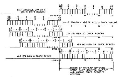
Fig. 13 Demonstration of correlation operation (The output resulting from the correlation operation is given in Fig. 11)
