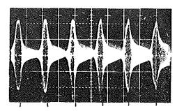
75 225 375 525 675 825 KHz lg. 28 Swept frequency response, Butterworth filter, taps 6 and 12.  $f_{\rm S}=900~{\rm KHz}.$
