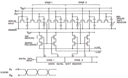
Fig. 2 The Binary Analog Correlator made using Metal-Oxide-Silicon Integrated Circuit Technology.
