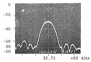
Fig. 20 Bandpass response corresponding to impulse response of Figure 19.
