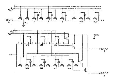
Fig. 11 Equivalent circuit diagram for an audio-frequency BBD, the SAD-1024.
