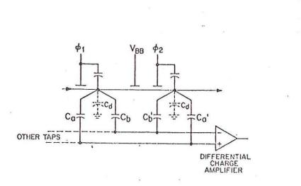
Fig. 9 Capacitive divider taps for BBD.
