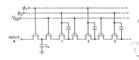
Figure 2. Improved Bucket-brigade Structure With Tetrode Isolation
