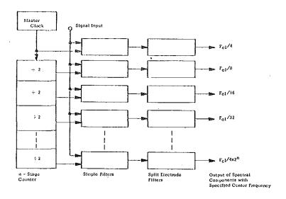
Figure 17. Spectrum Analyzer Using Transversal Filters.
