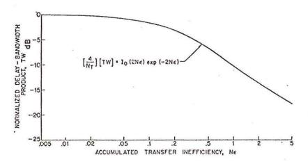
Fig. 5 Normalized delay-bandwidth product vs. accumulated transfer inefficiency NE.
