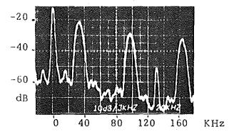
g. 22 Bandpass response corresponding to impulse response of Figure 19, scan extended to area of sampling frequency.
