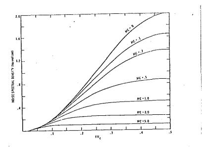
Fig. 6. Normalized noise power spectral density as a function of normalized frequency. Imperfect charge transfer severely attenuates the high frequency noise components.
