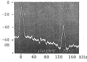
Fig. 9 Spectral response as in Figure 8, extended to show sampling-frequency area.
