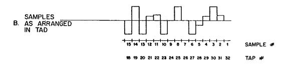
Figure 7. Arrangement of Samples of Input Chirp Along the Length of a Tapped Analog Delay.
