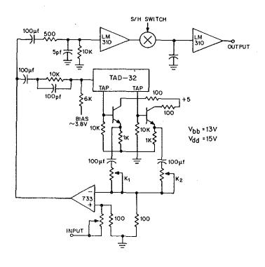
Fig. 25 Circuit diagram of experimental recursive filter.
