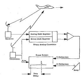
Figure 10. Radar Application for Binary Analog Correlator.
