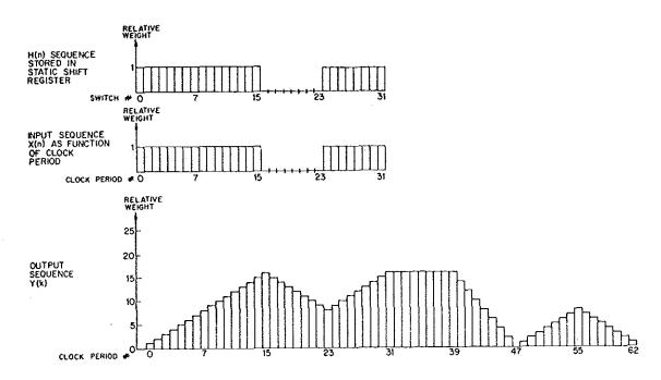
Fig. 3 Convolution of two-valued (bi-phase) sequences
