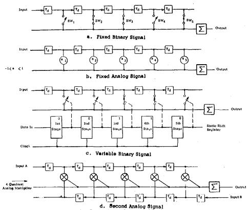
Figure 2. Comparison of Various CTD Structures.
