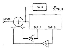
Fig. 24 Block diagram of experimental recursive filter.
