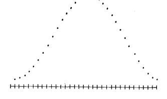
Fig. 6 Hamming window for 32-tap filter an oscilloscope overlay.
