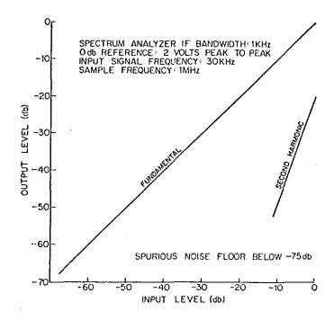
Fig. 7 Dynamic range and linearity for tetrode BBD.
