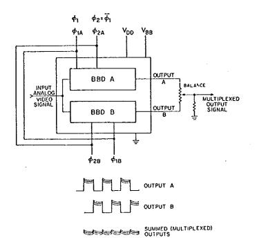
Fig. 12 Method of multiplexing delay lines to obtain wide-band high-frequency operation (SAD-341).
