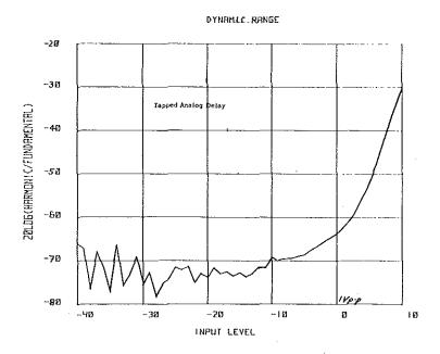
Figure 5. Harmonic Distortion of Tapped Analog Delay.
