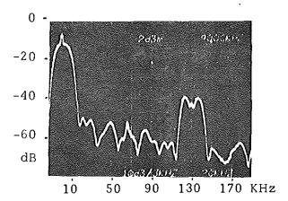
Fig. 15 Frequency spectrum, wide band, scan extended to show sampling-frequency rate.
