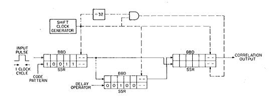
Fig. 14 Simulation of autocorrelation experiment using the Binary Analog Correlator as code generator, delay simulator and auto correlator.
