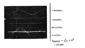
Figure 13. Demonstration of Convolution/Correlation Performed by Analog Analog Correlator.
