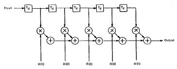
Figure 1. General Symbolic Representation of a Discrete-Time Signal Processing Device.
