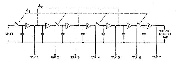
Figure 1: A Tapped Analog Delay Line Made with Sample and Holds.
