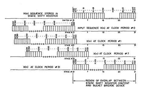
Fig. 5 Demonstration of the convolution operation (The output resulting from the convolution operation is given in Fig. 3)
