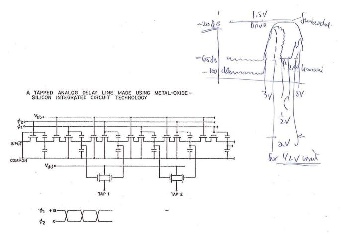
Fig. 8 Equivalent schematic circuit for tapped BBD.
