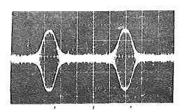
450 900 1350 KHz ig. 26 Swept frequency response, Butterworth filter, taps 1 and 2.  $f_S = 900 \, \text{KHz}$ , sweep 0 - 2 MHz.
