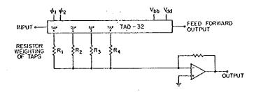
Fig. 13 The TAD-32, a Tapped Analog Delay device.
