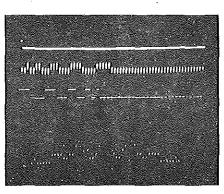
Fig. 15 Demonstration of correlation of simulated bi-phase chirp pattern with chirp pattern in static shift register.
