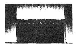
Fig. 3 Oscillogram of equal-weight impulse response.
