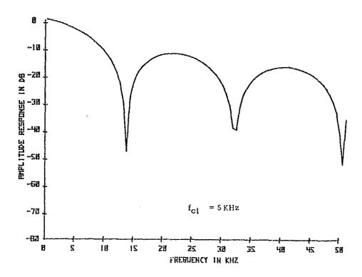
Fig. 7 Frequency spectrum of Binary Analog Correlator corresponding to a rectangular window of 32 taps.
