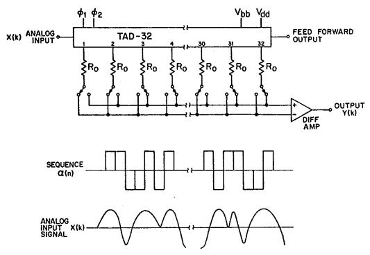
Figure 6. Schematic Showing the Tapped Analog Delay as a Bivalued Analog Correlator.
