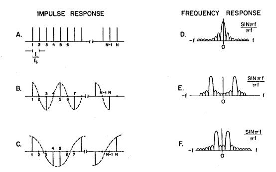
Figure 8. Three Simple Impulse Responses and the Resulting Frequency Response Produced by Each.
