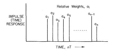
Fig. 2 Impulse response of FIR filter of Fig. 1. For uniform weighting, all  $a_i = 1$ .
