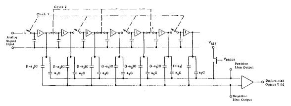
Figure 14. Transversal Filter with Split Electrode Structure.
