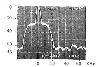
Fig. 16 Frequency spectrum, narrow band, corresponding to impulse response of Figure 13.
