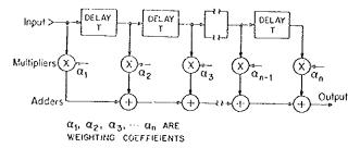
Fig. 1 General state diagram for transversal (FIR) filter.
