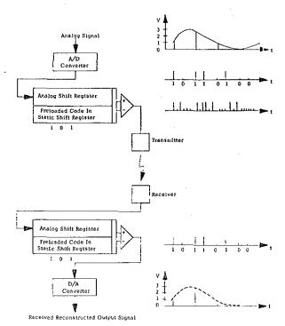
Figure 11. Binary Analog Correlator Used in Spread Spectrum Communication System.
