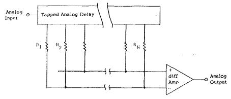
Figure 4. Tapped Analog Delay
