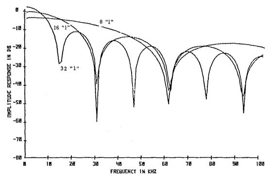
Fig. 8 Frequency spectrum of Binary Analog Correlator corresponding to windows of different widths.
