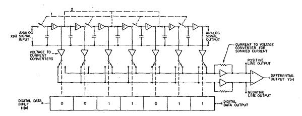
Fig. 1 A Binary Analog Correlator made with sample-and-holds and tapped-switches controlled by a static shift register.
