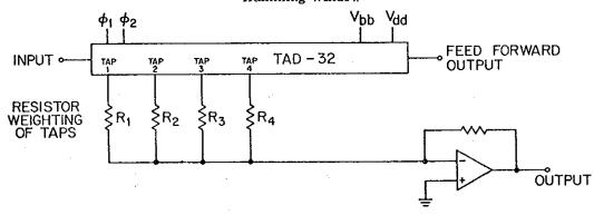
Figure 4. Schematic Representation Showing Resistor Loading of Taps for the Realization of a Desired Filter Function.
