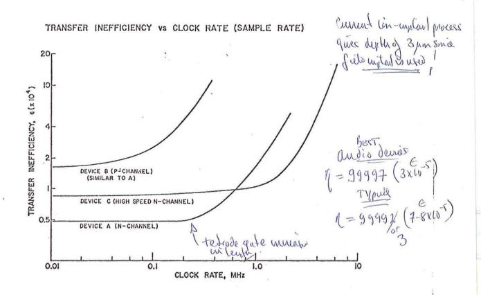
Fig. 4 Transfer efficiency vs. sample rate for two commercial audio devices and one high-speed device.
