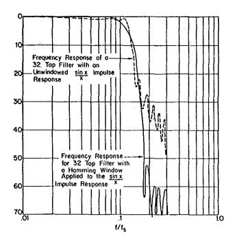
Figure 10. Comparison of Window and Unwindow Filter Response.
