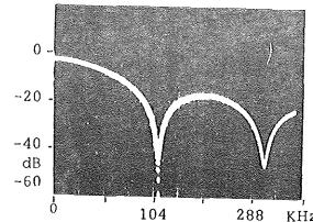
Fig. 5 Frequency spectrum for equal-weight FIR filter; 3 Hz resolution bandwidth, 360 KHz scan.
