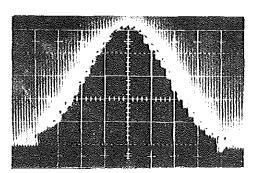
Fig. 7 Impulse response with equal weighting modified by Hamming window.
