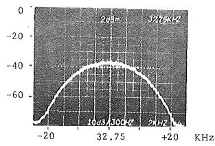
Fig. 21 Center section of Figure 20 expanded to show rounded passband shape.
