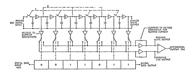
Fig. 14 An example of a BBD Binary-Analog Correlator (BAC-32).
