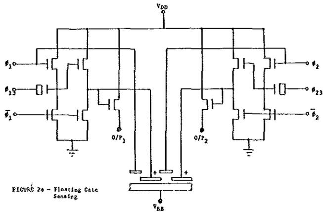
FIGURE 2a - Floating Gate Sensing
