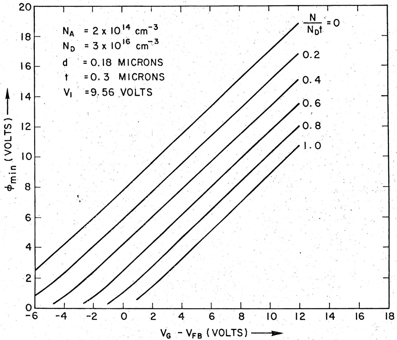
Fig. 2. Minimum potential vs. gate voltage for an implanted-channel CCD.
