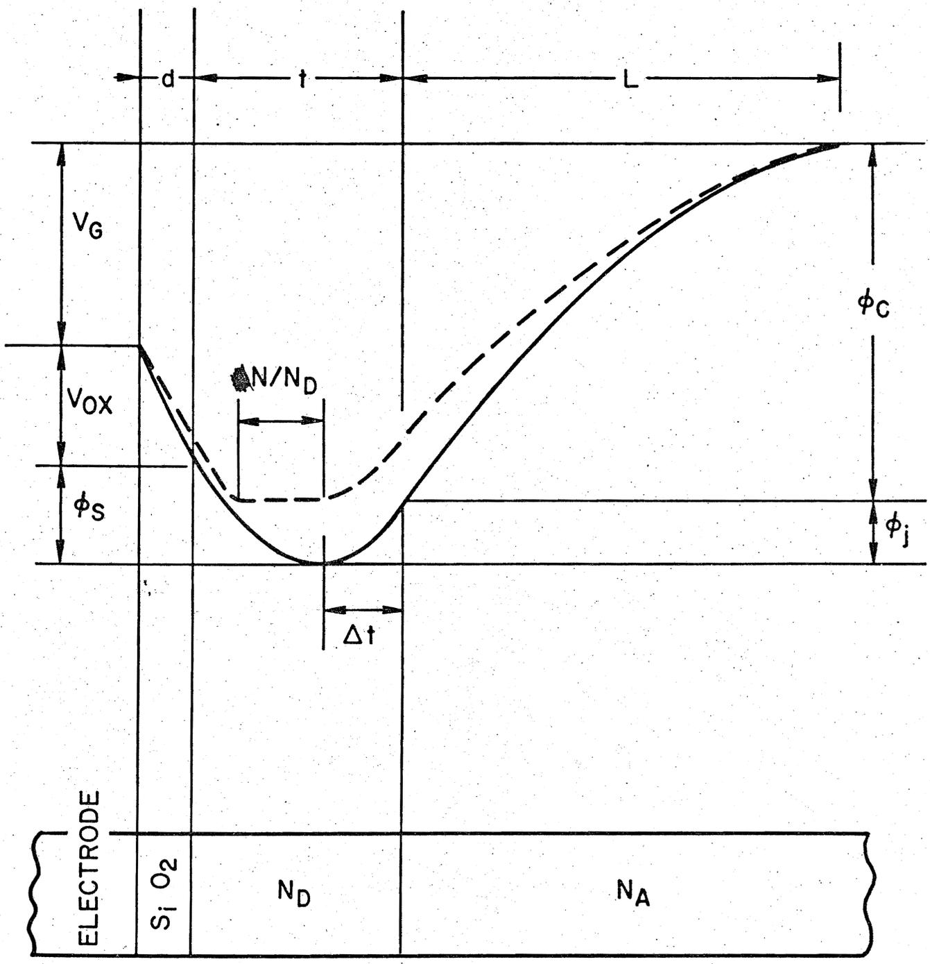
Fig. 1. Potential profile of buried channel CCD
