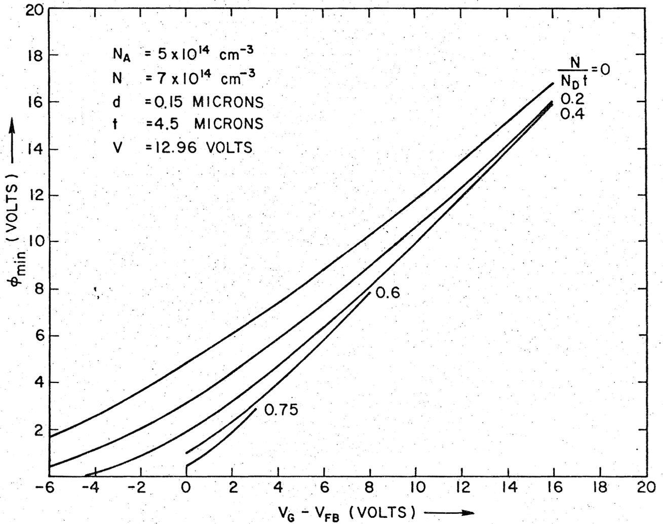
Fig. 3. Minimum potential vs. gate voltage for an epitaxial-channel CCD.
