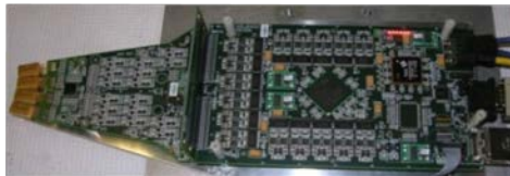
64-channels front-end board and digitizer
