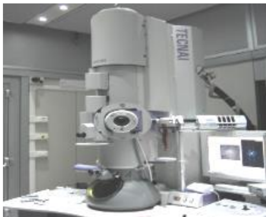
TEM/STEM: TECNAI G2 F30 S-Twin equipped with Lorentz Lens, Bi-prism. EELS and EDX detector. Holography, Tomography
