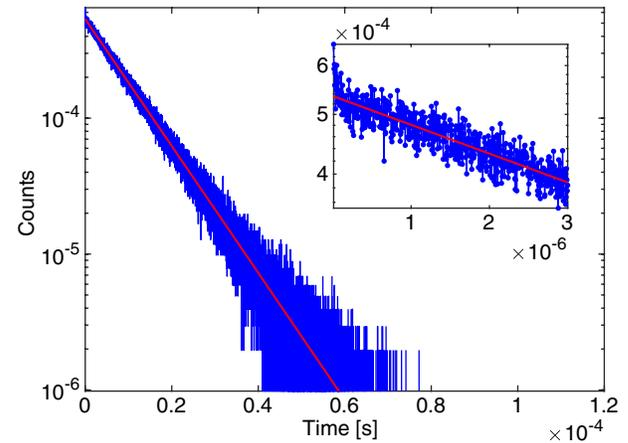
Fig. 8. Inter-pulse time distribution of the bottom SPAD when average count rate is  $100\text{ kcps}$ . The red line shows the fitted distribution. The inset is a zoom on shorter time intervals.
