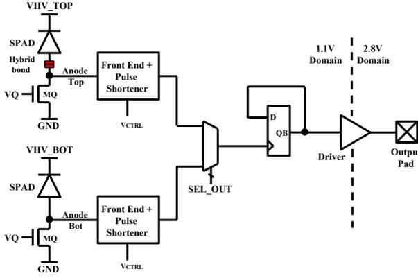
Fig. 2. Circuit diagram of the dual layer SPAD pixel.
