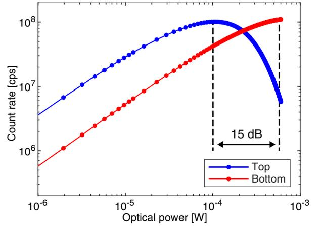
Fig. 4. Count rate versus optical power at 2 V excess bias.
