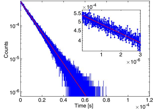
Fig. 7. Inter-pulse time distribution of the top SPAD when average count rate is  $100\text{ kcps}$ . The red line shows the fitted distribution. The inset is a zoom on shorter time intervals.
