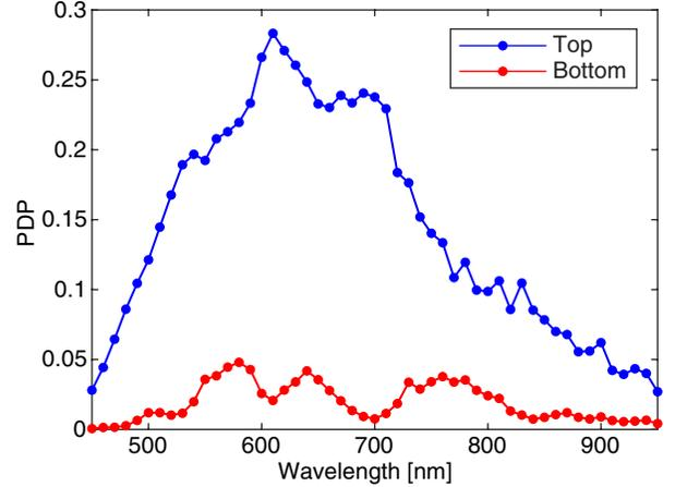
Fig. 3. Photon detection probability at excess bias of 3 V, wavelength step of 2 nm, and bandwidth of  $\sim 2 nm$ .
