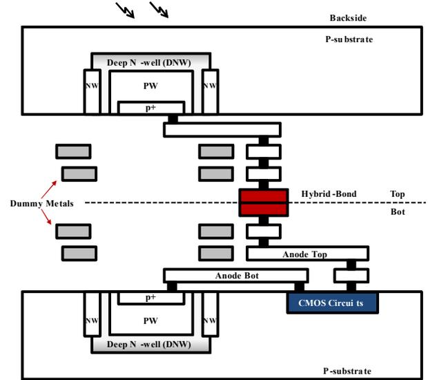
Fig. 1. Cross-section of the dual layer SPAD pixel.
