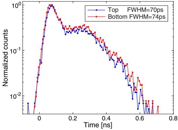
Fig. 5. The jitter histogram for the top and bottom SPADs at excess bias of  $2V$ , and wavelength of  $773\text{ nm}$ .
