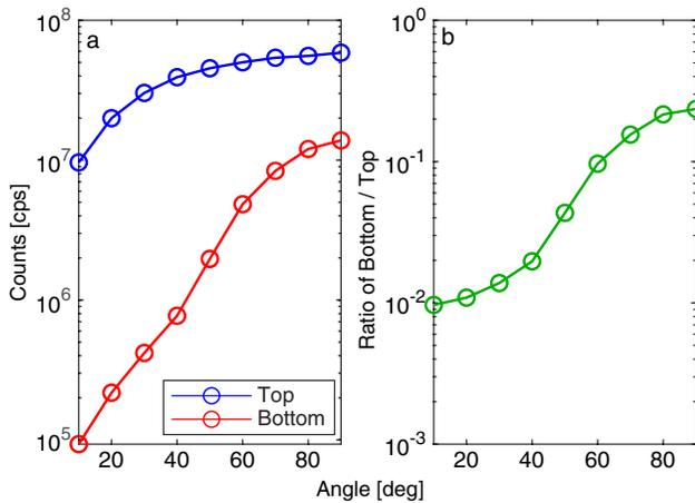
Fig. 10. The effect of incident light angle on (a) Count rate (b) Ratio of bottom to top SPAD count rates.
