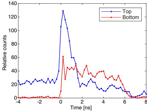
Fig. 6. The recovery of a  $6\text{ ns}$  laser pulse under pile-up conditions.
