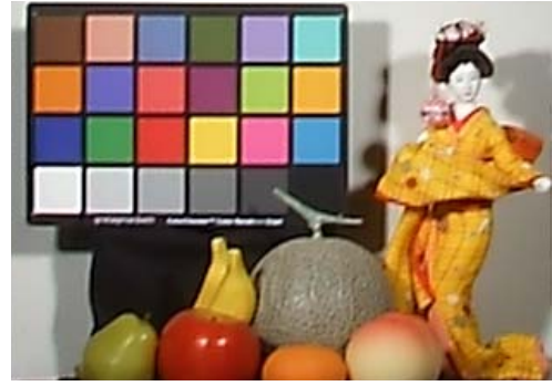
Fig. 8 Photograph of a Japanese doll with a Macbeth chart, which was taken by a trial product of the proposed CMOS sensor with micro-color filters.
