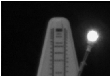
Fig. 6 Photograph of an operating metronome, which was taken by a trial product of the proposed CMOS sensor without micro-color filters.
