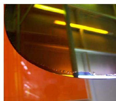
Optimization of bonding and grinding process to eliminate edge-cracking during subsequent processing
