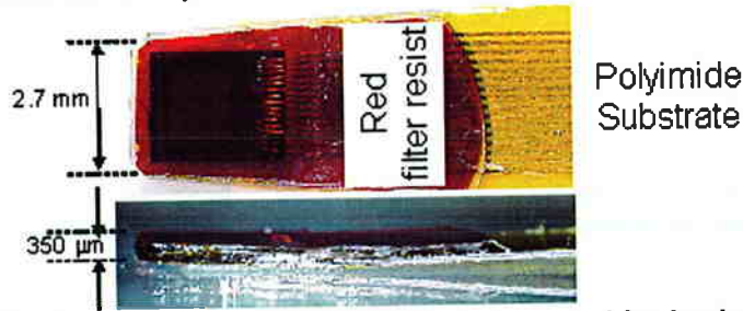
Figure 5: 176x144-pixels (QCIF) image sensor assembled for in vivo applications
