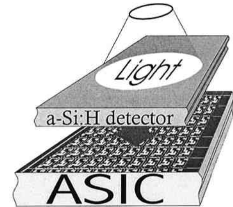
Fig. 1 Principle of TFA technology
