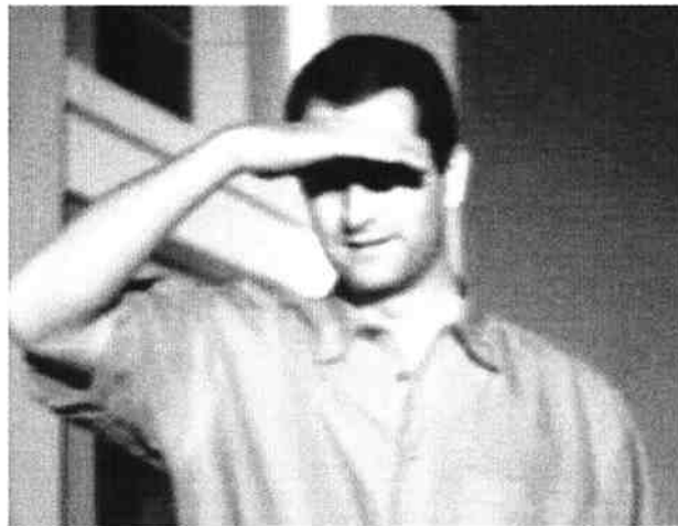
Figure 1: These three images were captured using the FFOA high sensitivity sensor at identical frame rates (60 fps) and iris settings ( F= 1:1.4 ). The scene illumination in the top image was 0.2 Lux. The center image illumination was 200 Lux and the final illumination was greater than 20,000 Lux (bright sunlight).
