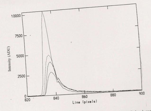
The ability of the charge packet to survive the readout process in a radiation damaged CCD is strongly a function of the charge filling the rest of the image area. If the rest of the pixels have a large amount of charge in them, then their traps are filled, and the probability of an electron in a charge packet encountering an empty trap decreases.
