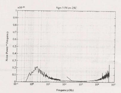
Damaged MOSFET noise spectra were recorded as a function of temperature and subsequently separated into their constituent components: Johnson noise, flicker (1/f) noise and ge-re noise. It was found that most spectra clearly contained ge-re noise from a small number of ge-re centres.
