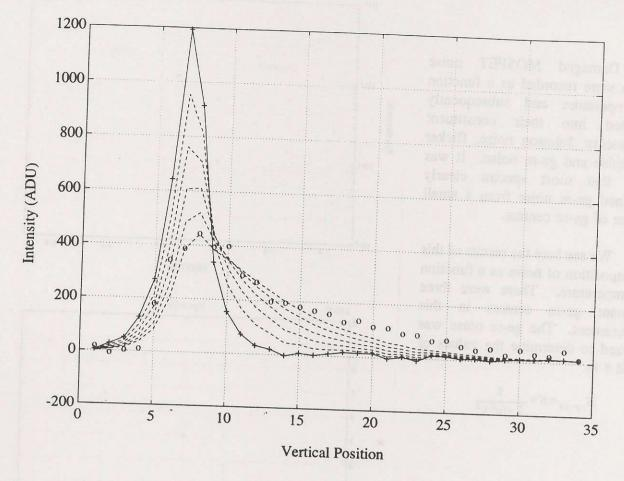
Trapping in the imaging area of a CCD causes losses both through image deferral (charge packet deferral) and image loss. We investigated both of these degradations in a radiation damaged CCD.
