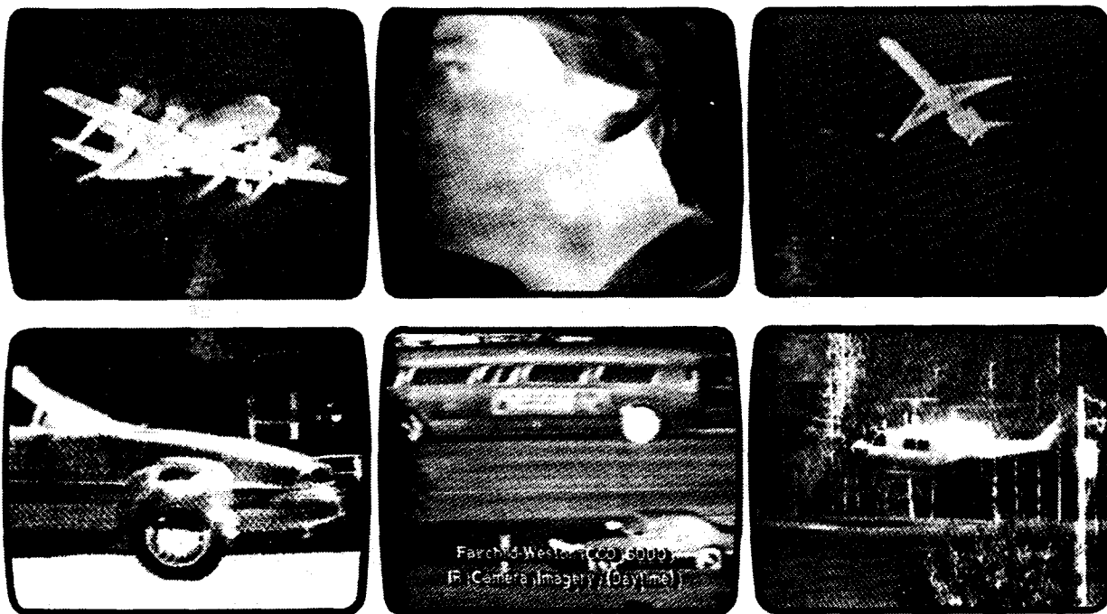
Fig. 16. Thermal imaging obtained with Fairchild 512 x 488 FPA.
