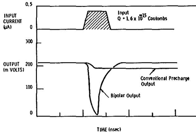
Figure 2(b) SPICE simulation of the bipolar output. The response to a current pulse  $I_B$  is shown. This simulation is more optimistic than the charge control theory because default parameters for the bipolar are used.
