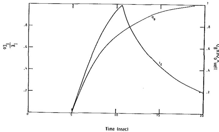
Figure 2(a) The emitter current response of the bipolar for a charge packet. The charge packet size ( $Q_{A_{well}} = 1.6fc$ ) and the maximum emitter current is  $I_{E0} = 2.3\mu A$ . The calculations are based on  $\beta=100$  and  $k=0.9nsec$ .
