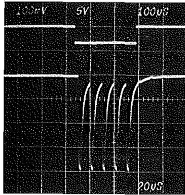
Figure 5 Input and output of a CCD shift register with a bipolar output.
