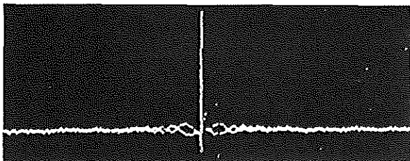
Figure 9(b) Matched Filter Response to 256-Point Chirp Waveform 0 - f_c/2 Hz (TB = 128)
