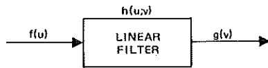
Fig. 1. General linear filter characterized by impulse h(u,v) . Input f(u) is transformed into output g(v) through a linear transformation integral.
