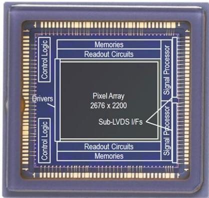
Fig. 8. Chip microphotograph
