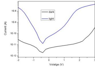
Figure 6. I-V curve of the photodetector pixel on the dummy chip
