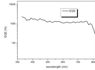
Figure 5. EQE vs. wavelength of the photodetector pixel on the dummy chip
