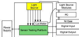
Figure 4. Illustration of measurement of photoelectric performance for perovskite CMOS chip
