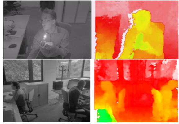
Fig. 7. Left sensor image and depth map sample image (frame rate 25Hz, exposure time 40ms)
