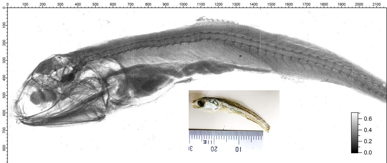
Fig. 7 An X-ray projection image of a dried sardine taken by a conventional micro-focus X-ray source with a Cu target at the operation of 40 kV 0.8 mA. Background and flat field calibration was carried out. Exposure time of 1 sec, and a projection magnification of 2 were used. Inset shows the optical image of the sample.
