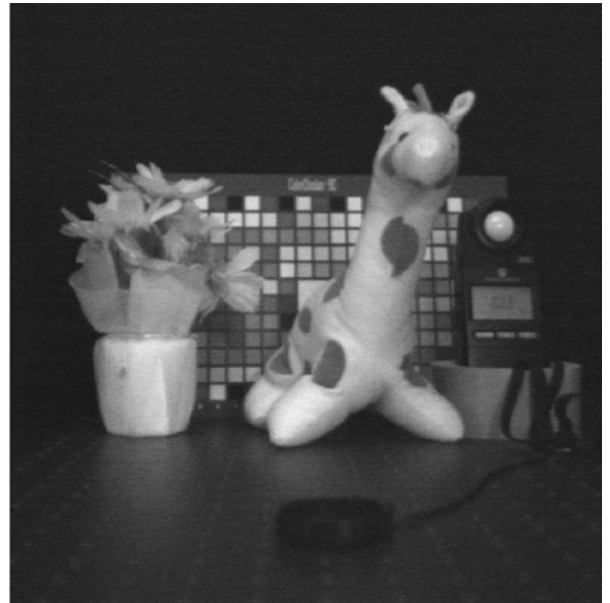
Fig. 8 Sample image (1M pixels) at low light level measured with a 1Mpixel CMOS imager ( F=1.4 , 4300K with IR cut filter, 10fps, 0.03lx).
