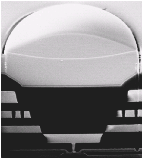
Figure 3 – Germanium diode embedded in CMOS
