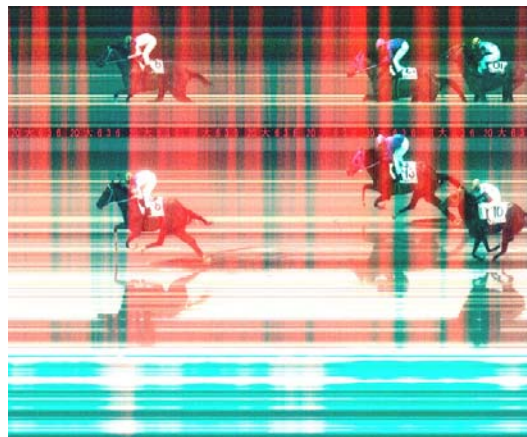
Fig.9. Race track camera image with conventional CCD.
