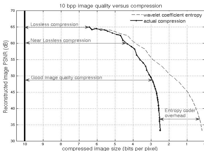
Figure 7: Reconstruction PSNR vs. image compression for a Bayer 3 MPix 10 bits cameraphone image (solid line).
