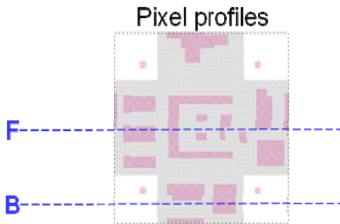
Figure 4. Layout of a preShape pixel from the TPAC1.0 sensor. Only the N-well (purple) and deep P-well (grey) layers are shown. Every N-well but the detecting diodes have got deep P-well underneath. The non-physical boundary between pixels is shown as a dotted line.
