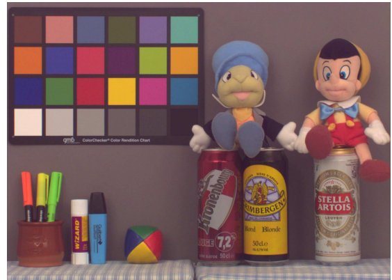
Figure 12: Image, taken with back-illuminated image sensor demonstrator in 1T5 architecture with 1.4µm pixel pitch, deep diode on n-substrate
