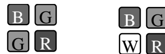
Fig. 1. 2 x 2 unit pixel blocks of the Bayer Pattern (left) and the newly developed the Bayer-like WRGB Pattern (right).
