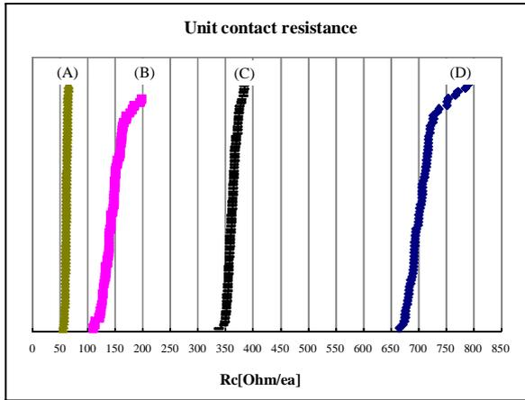
Fig. 3. Comparison graph of metal 1 contact resistance
