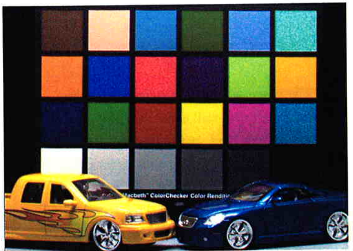
Figure 10. Color Image from 900x640 pixel array with 1.7um pixel size
