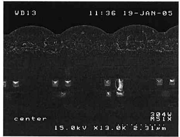
Fig. 3: Cross section of interconnect stack with nitrides removed in the optical path.
