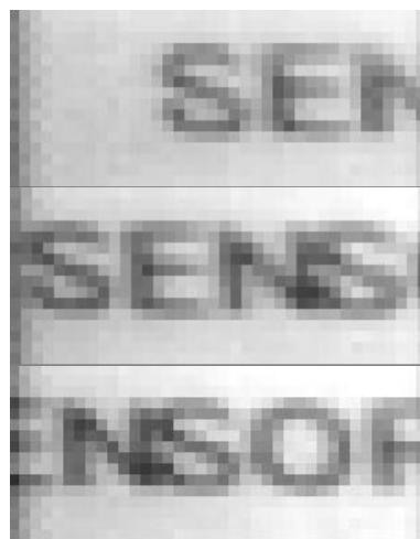
Fig. 7. Analog output images obtained by the first prototype (characters of "sensor" are moving.)
