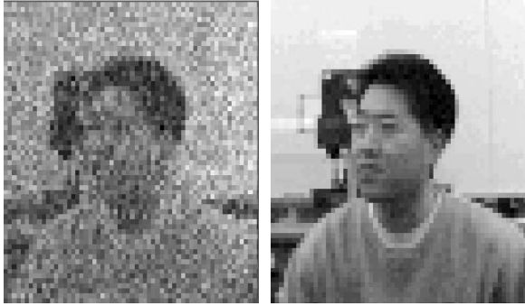
Figure 6. (a) Raw image captured under room light of approximately 200 lux. (b) Image corrected by subtraction of a white image
