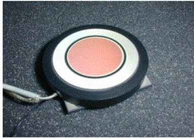
Figure 1: The Multi-pixel Hybrid Photo Diode
