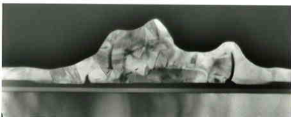
Fig. 6 TEM of a SiP precipitate with X-ray mappings of Si and P
