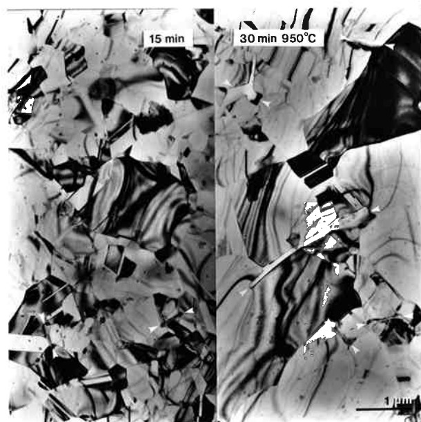
Fig. 4. Plan-view TEM images of \text{POCl}_3 -doped poly-Si at 950^\circ\text{C} for 15 and 30 minutes. SiP precipitates are indicated by white arrows.
