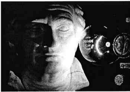
Fig. 8 High contrast scene captured with short integration time
