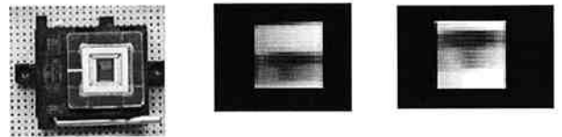
Figure 7: The prototype chip. And the obtained images(middle and right) when "T" is moving up and down and projected on the focal plane.
